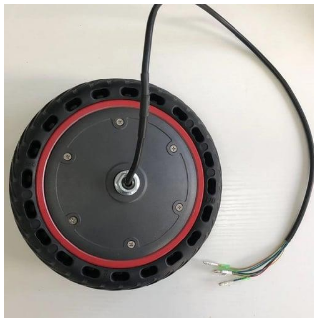
Figure 25: Electric Scooter Front Wheel containing the motor. [6]
